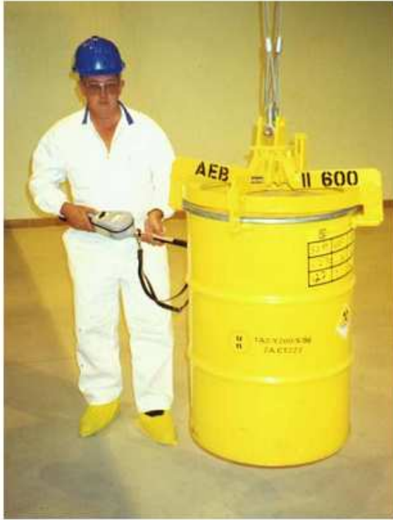
Figure 3-7: Standard steel and concrete containers used for radioactive waste disposal at Vaalputs
