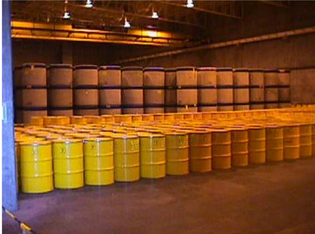
Figure 3-8: Storage facility for ILW and LLW showing concrete drums in the background and steel drums in the foreground
