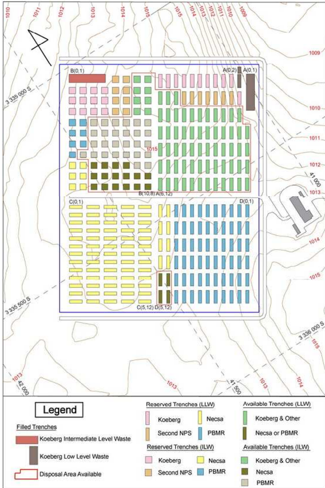
Figure 3-9: Trench layout for low and intermediate level waste at Vaalputs (Aquisim 2008)
