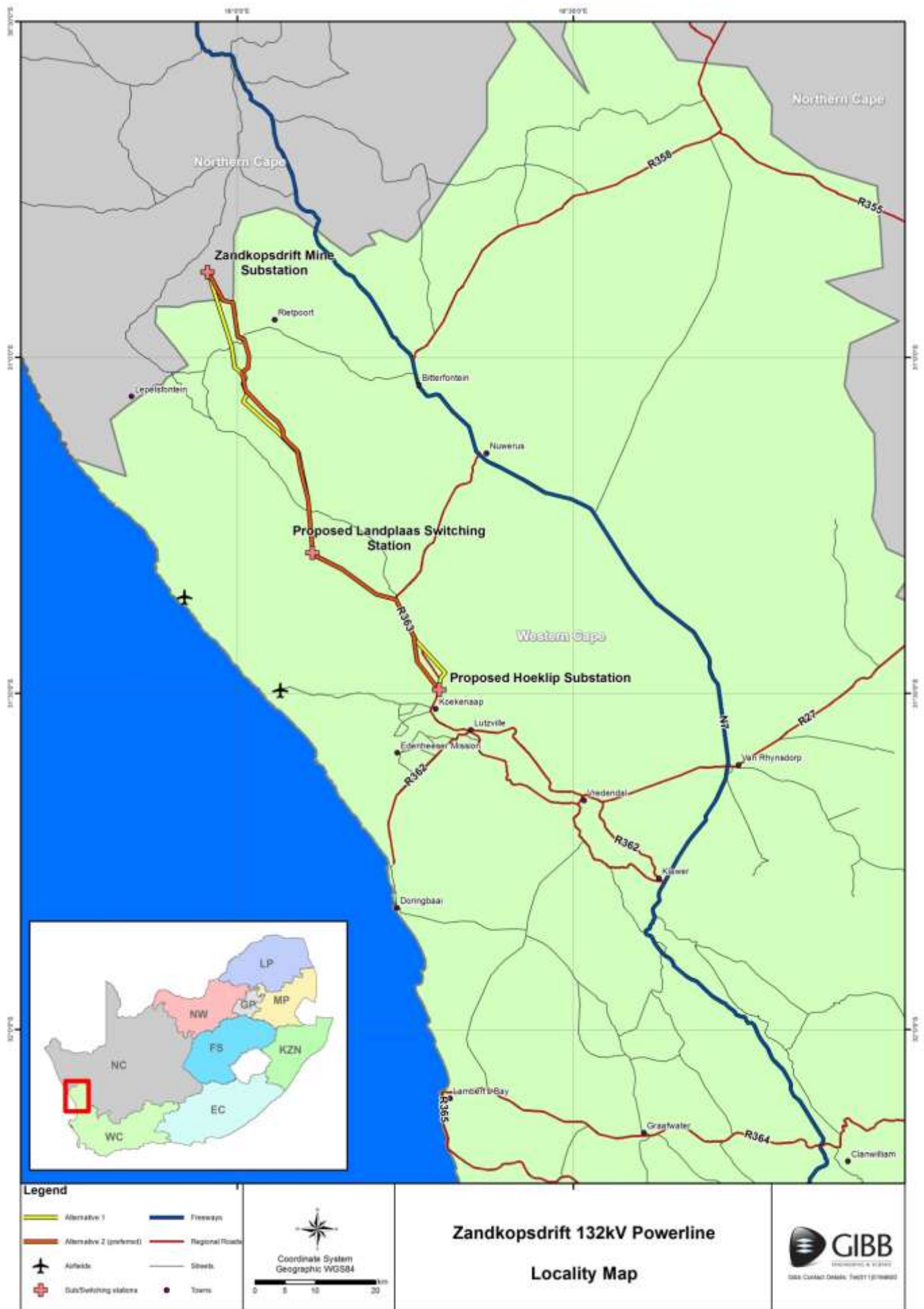
Figure 1: Alternative 1 & 2 distribution line alignments
