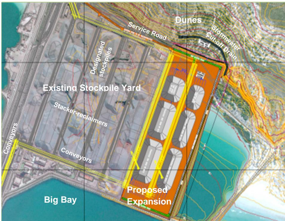
**Figure 9:** Layout of proposed Stock Yard Extension
