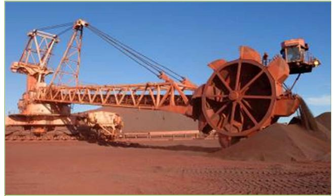
**Figure 10:** Photographs of a typical stacker-reclaimer
