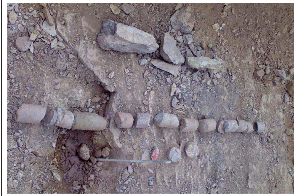
Figure 3: Intact rock condition encountered in trial drilling of a siliceous mudstone.
