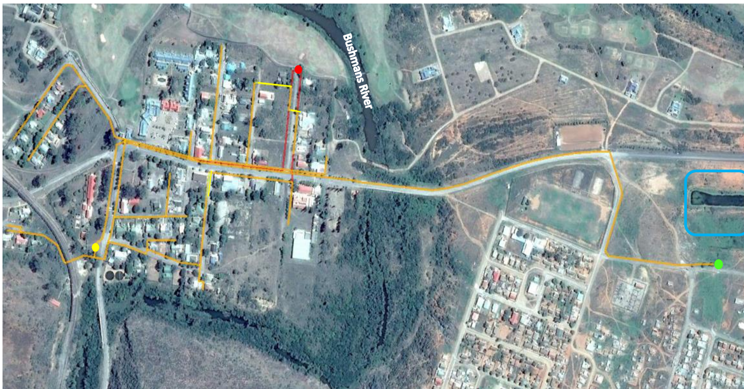
Figure 1: Proposed sewerage upgrade in Alicedale showing gravity lines and rising main common to Alternative 1 and 2 (orange lines), pump station 1 (yellow dot), pump station 2 (red dot), and connection to the gravity main (green dot). Where Alternative 1 pipeline differs from Alternative 2 this is shown as a yellow line. Where Alternative 2 pipeline differs from Alternative 1 this is shown as a red line. The historic detention pond that is listed as an NFEPA (2011) wetland is indicated in blue.
