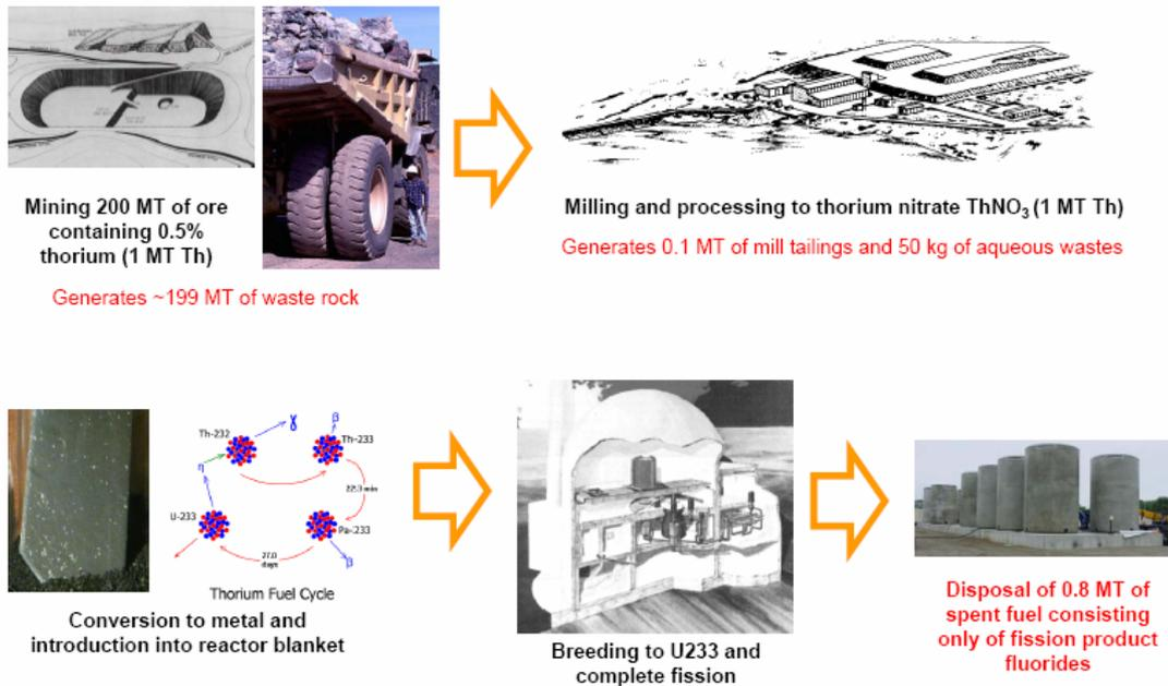
Thorium mining calculation based on data from ORNL/TM-6474: Environmental Assessment of Alternate FBR Fuels: Thorium
