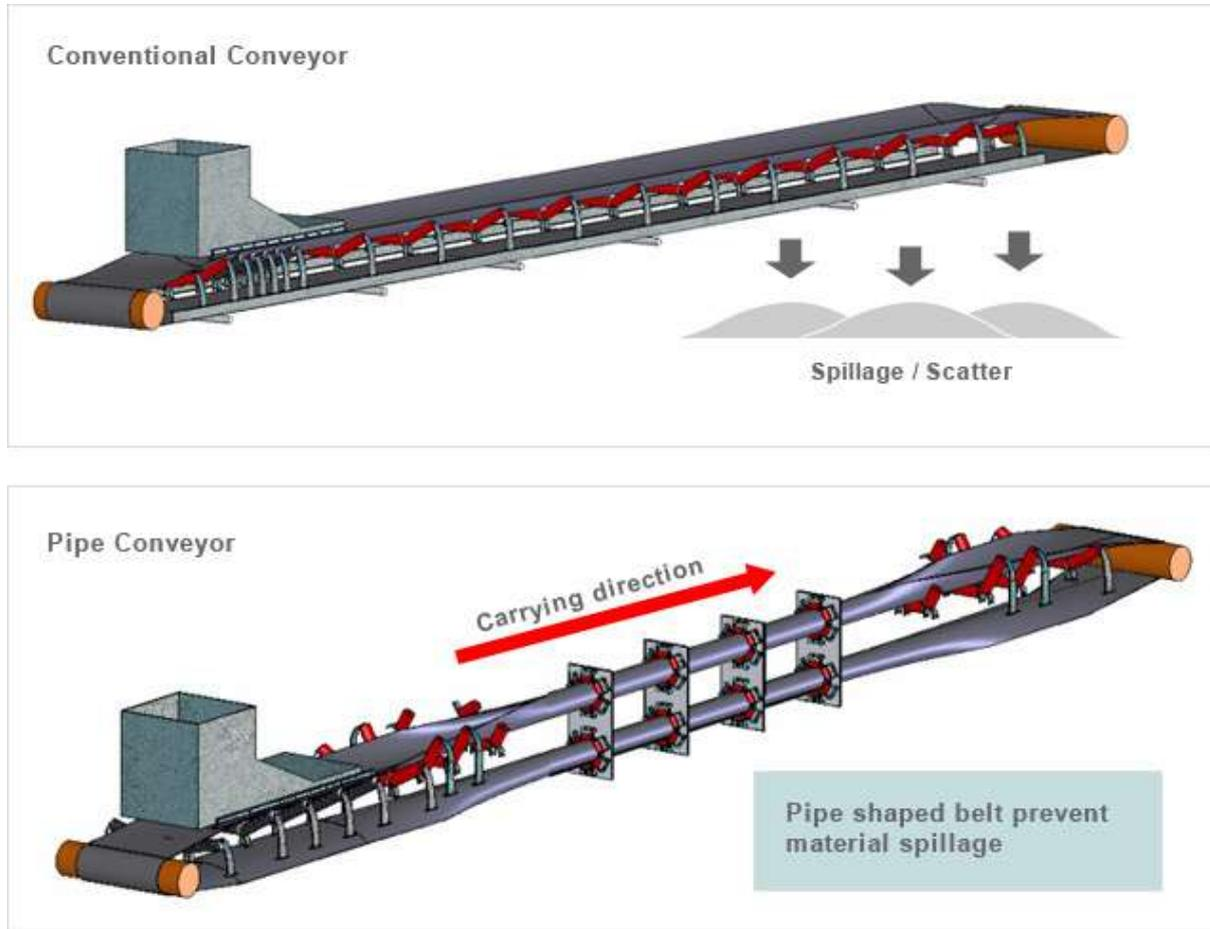
Figure 2: Example of a conventional conveyor in relation to a pipe conveyor (after Bridgestone, [http://www.bridgestone.com/products/diversified/conveyorbelt/products/pipe\\_conveyor\\_belt.html](http://www.bridgestone.com/products/diversified/conveyorbelt/products/pipe_conveyor_belt.html))
